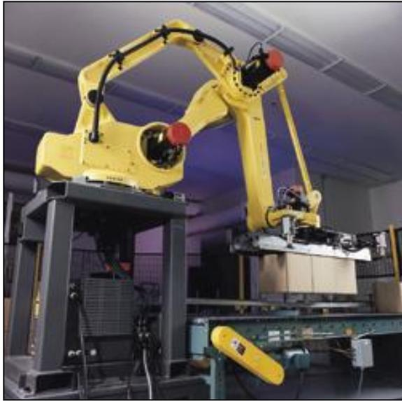
**Robot used to palletize cartons**
