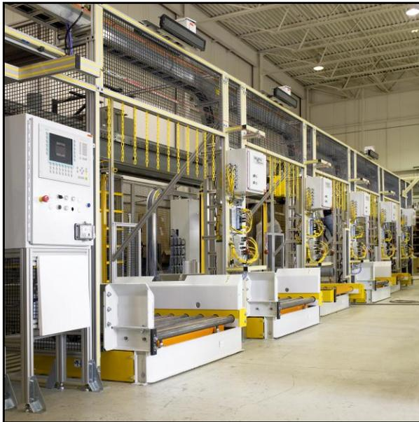
Creative Automation Inc. has experience in designing and building small pick and place systems for loading small parts into totes, to the large system shown on this page that loads and unloads Transmission Cases from pallets.
