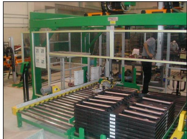
**Gantry palletizer for automotive camshaft blanks**
