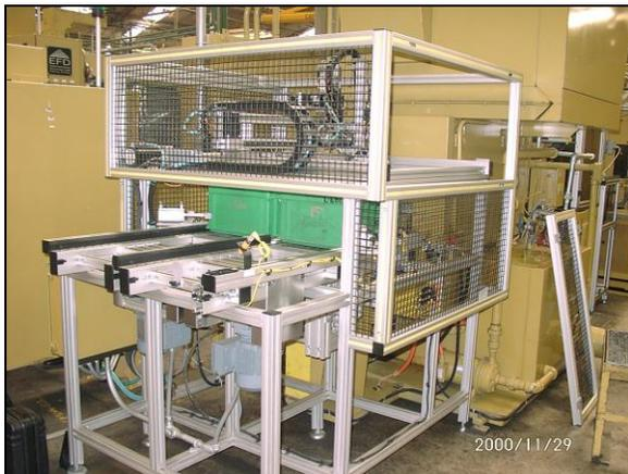
**Pick and place palletizer used to place small shafts into tote bins**
